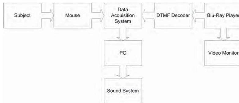
**Fig. 4.** A block diagram of the CMM simulator.
