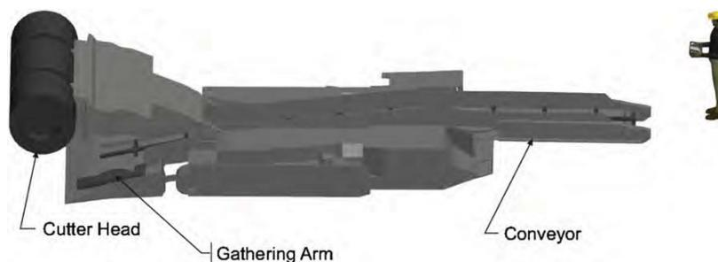
**Fig. 1.** Depiction of the CMM and operator relationship – the miner operator stands at the rear and operates the CMM by remote control. The cutter head cuts the coal which is then “swept” onto a conveyor by gathering arms. Coal exits the rear of the conveyor onto a shuttle car (not shown) that transports the coal. The conveyor boom can swing left or right as needed.
