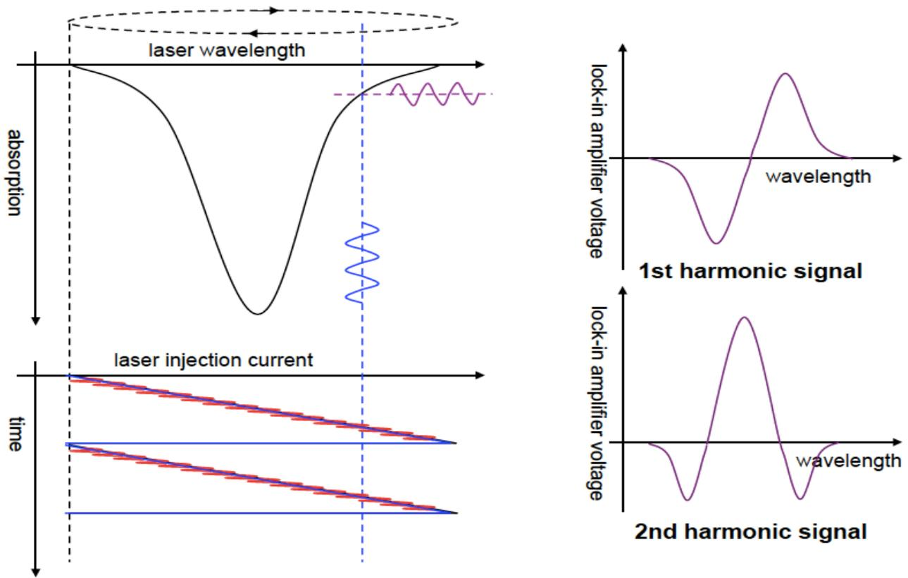
Fig. 4 – Principle of operations – wavelength modulation
