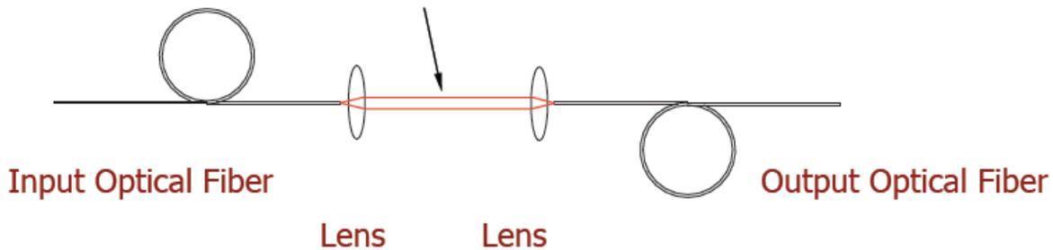
Fig. 1b – Remote Optical Methane Detector
