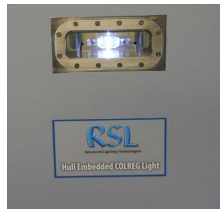
Figure 5: Navigation Luminaire Flush with Exterior Surface
