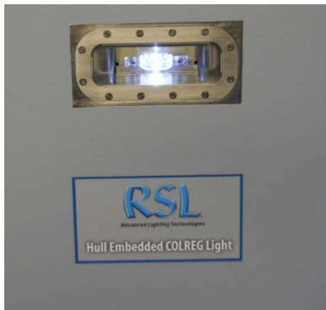
Figure 5: Navigation Luminaire Flush with Exterior Surface
