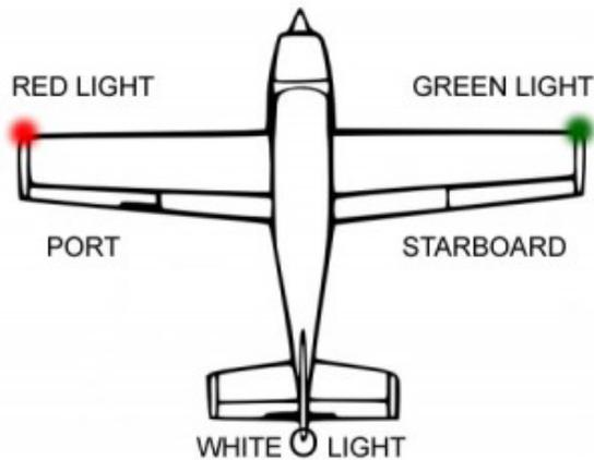
**Figure 3: Aircraft Position Lights** <sup>(4)</sup>
