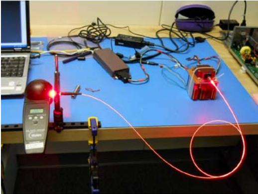
**Figure 1: Red Laser Luminous Flux Test Set Up**
