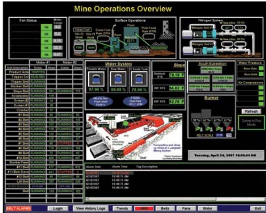
Figure 4: Typical Mine Wide Control and Monitoring System – HMI (© Pillar Innovations)
