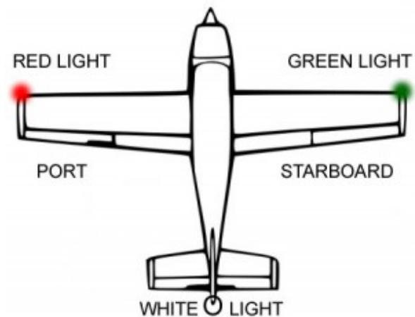
**Figure 3: Aircraft Position Lights <sup>(3)</sup>**
