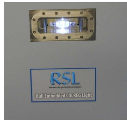
**Figure 5: Navigation Luminaire Flush with Exterior Surface**
