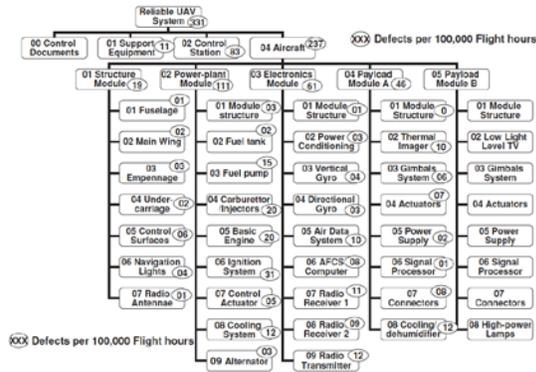
Fig. 14– UAV System Reliability Hierarchy
