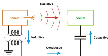
Fig. 10 - Typical EMI coupling mechanisms with source being a “noisy” navigation or strobe light and victim being a nearby sensitive digital/RF hardware or antenna.
