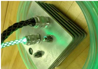
Fig. 2 – Encapsulated Light Engine
